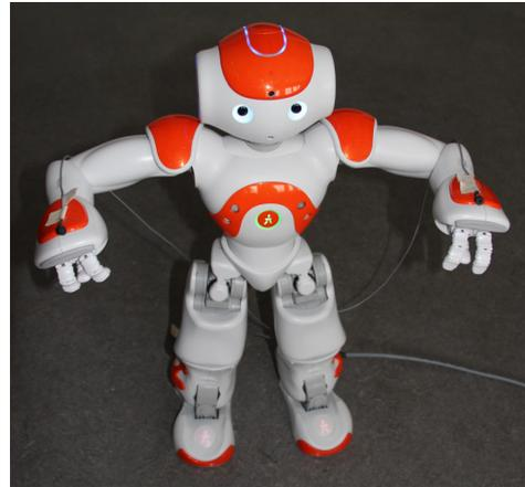
**Figure 1:** NAO H25 robot with additional peripheral capsule microphones (AKG CE 20/17) attached on the back of its hands. The height of this robot is 573 mm and the shoulder-to-shoulder length is 275 mm.
