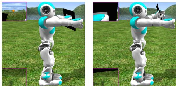
Fig. 1. The simulated experimental setup. The robot is holding a shield in its left hand and is facing an object. In the left image, the configuration of the robot's arm does not hide the orange ball situated in front of the robot (the visual input from the robot's top camera is visible in the upper left corner of the image). In the right image, the configuration of the arm results in a full occlusion of the object, as visible from the robot's top camera.
