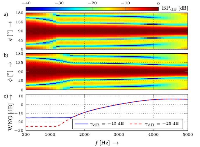
**Fig. 2.** Design example of free-field-based RLSFI beamformer for a five-element microphone array. Beampatterns for WNG constraints a)  $\gamma_{\text{dB}} = -25 \text{ dB}$  and b)  $\gamma_{\text{dB}} = -15 \text{ dB}$ . The resulting WNG in illustrated in c).
