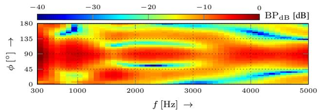
**Fig. 3.** Illustration of the beampattern in dB of the five-element free-field-based RLSFI beamformer with WNG constraint  $\gamma_{\text{dB}} = -15 \text{ dB}$ , computed with HRTFs as sensor responses  $g_n(\omega, \phi, \theta)$ .
