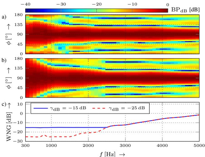
**Fig. 4.** Design example of HRTF-based RLSFI beamformer for a five-element microphone array. Beampatterns for WNG constraints a)  $\gamma_{\text{dB}} = -25$  dB and b)  $\gamma_{\text{dB}} = -15$  dB. The resulting WNG is illustrated in c).
