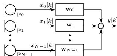
Fig. 1. Illustration of filter-and-sum beamforming [6].
