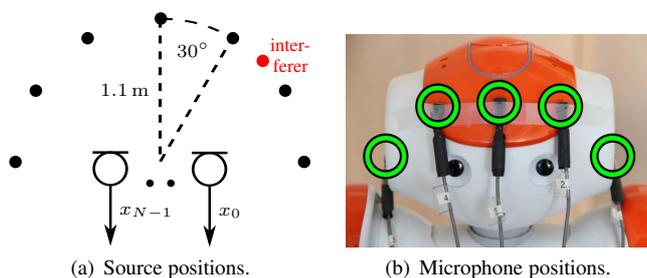
**Fig. 6.** Illustration of evaluated source positions and the employed microphone positions at the robot's head.
