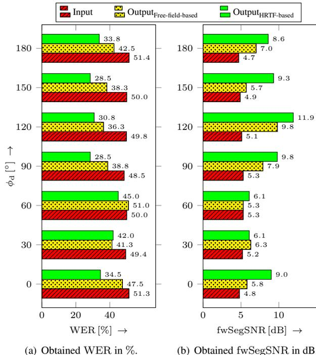
**Fig. 7.** Illustration of WERs in % and fwSegSNR levels in dB, obtained at the input and at the output of the free-field- and HRTF-based beamformers.
