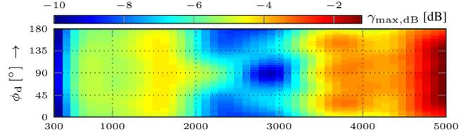
**Fig. 5.** Illustration of maximum possible WNG  $\gamma_{\text{max}}(\omega_p)$  for the HRTF-based beamformer design. In general, a lower maximum WNG is obtained than for the free-field design.
