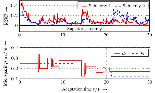
**Fig. 8.** Illustration of array topology adaptation for  $\phi_{\text{int}} = 40^\circ$  and  $T_{60} \approx 100$  ms.
