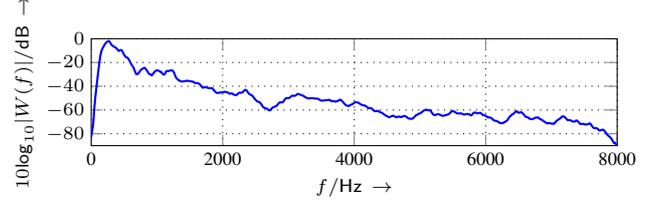
Fig. 4. Example of an average speech PSD used as window function (5) in (4).
