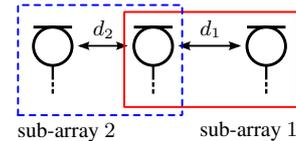
**Fig. 3.** Illustration of the employed sub-arrays for the case of a three-sensor linear array.
