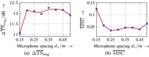
**Fig. 7.** Comparison of  $\text{SIR}_{\text{mean}}$  and  $\overline{\text{MSC}}$  obtained from sub-array 1 for different microphone spacings.
