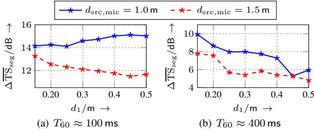
**Fig. 6.** Comparison of obtained target suppression performance  $\Delta\overline{\text{TS}}_{\text{seg}}$  in dB of the employed GC-BSS two-channel system for varying microphone spacings  $d_1$  and different source-microphone distances  $d_{\text{src,mic}}$  in two different acoustic environments.
