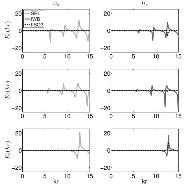
Figure 3. Dispersion error,  $E_n$ , shown for a plane wave incident axially (left column) and diagonally (right column), and for orders  $n = 0$  (top row),  $n = 2$  (middle row) and  $n = 8$  (bottom row). SRL - Standard rectilinear, IWB - Interpolated wideband, IISO2 - Interpolated isotropic.
