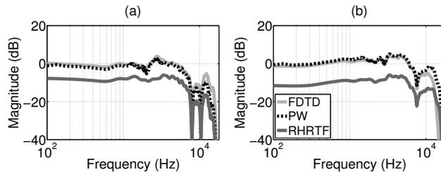
Figure 4. Magnitude of a left-ear binaural response shown for (a) incidence angle of  $\Omega = (\frac{\pi}{2}, 0)$  and (b) incidence angle of  $\Omega = (\frac{\pi}{2}, \frac{\pi}{4})$ . FDTD - finite difference simulation, PW - plane-wave closed form solution, RHRTF - reduced order HRTF (scaled down by 6dB for visual clarity). All results computed with (or reduced to)  $N = 12$ .
