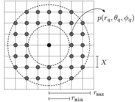
Figure 1. A 2D section of a volumetric shell array.  $r_{\max}$  and  $r_{\min}$  are the shell's outer and inner radii respectively, and the FDTD spatial period,  $X$ , controls the density of the receivers within the array.
