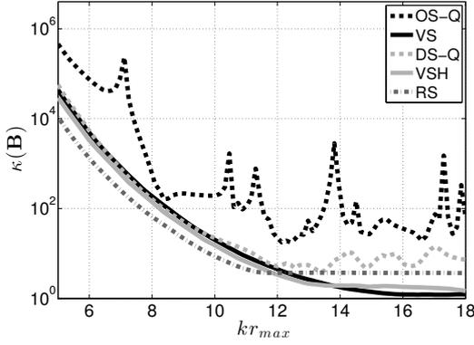
Figure 2. Condition number of a matrix  $\mathbf{B}$  as function of  $kr_{\max}$  shown for a number array configurations designed on an FDTD grid of sample period  $X = 10\text{mm}$ . In all cases, the matrix  $\mathbf{B}$  is computed with  $N = 12$ .
